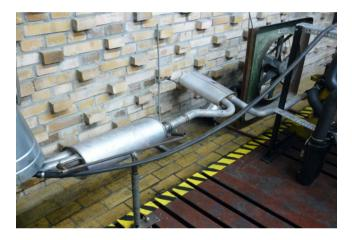
Figure 3. 13. The exhaust system of a combustion engine
