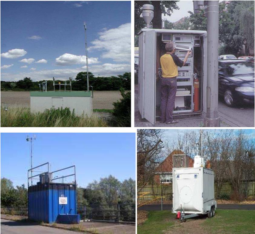
FIGURE 42 Different types of monitoring stations.
