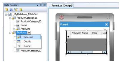
Figure 3-8 Automatic generation of DataGrid user interface assigned to Products DataSet
