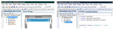
Figure 3-3 Creating Smart Device project type from existing code "FormHello.cs"
