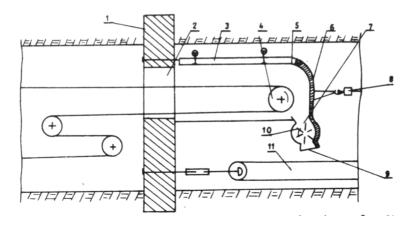
Fig.8.34. An air stopping over the belt conveyor (Wacławik et al, 1996) 1. stopping; 2. window; 3. hermetic shield; 4. conveyor; 5. joints; 6. front wall; 7. trough; 8. counterweight; 9. packing; 10. closure; 11. conveyor
