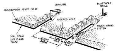
Fig.6.23. Auger hole patterns and effect of highwall curvature (after Treuhaft, 1984)
