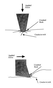
Fig.3.1. Methods of rock loading by an indenter (top) and a drag bit (bottom) (after Hood and Roxborough, 1992)
