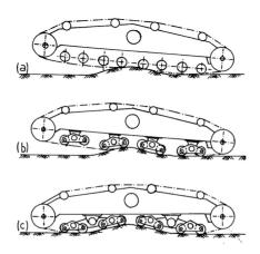
Fig.5.25. Continuous excavator crawlers (after Atkinson, 1992)
