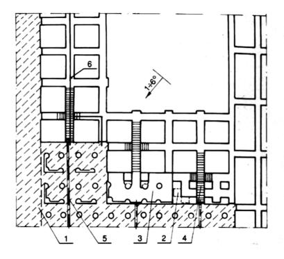
Fig.8.14. Two-phase, two-layer room-and-pillar method with hydraulic backfill (after Cieślik et al, 1991) 1. backfill; 2.upper layer mining; 3. lower layer mining ; 4. inclined drift; 5. dewatering collectors; 6. stowing pipeline
