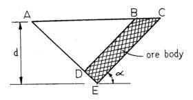
Fig.5.4. Overall stripping ratio representation (after Fourie, 1992)
