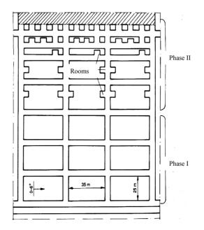
Fig.8.4. Two-phase room-and-pillar mining method (after Janowski et al, 1996)
