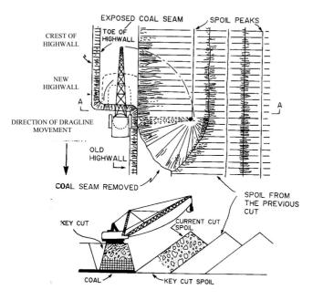
Fig.6.12. Simple side casting (after Bricker, 1992)
