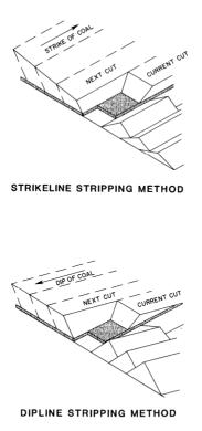
Fig.6.18. Stripping methods for dipping seams (after Stubblefield and Fish, 1992)
