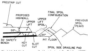
Fig.6.14. Multiple-pass, spoil-side stripping (after Bricker, 1992)
