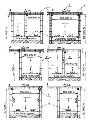
Fig.8.3. Types of mining panel development (after Janowski et al, 1996) 1. level roads; 2. inclines; 3. transfer point for the mined ore from underground haulers onto a belt conveyor; 4. transfer point for the mined ore from a belt conveyor onto the rail transport or main conveyor; 5. a conveyor flight; 6. haulage with underground haulers; 7. rail haulage
