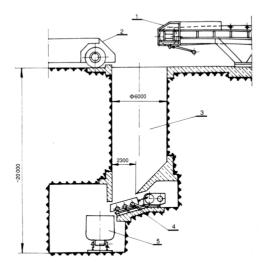
Fig.8.27. Surge bunker at loading point for mine rail cars (after Gładysiewicz and Pelc, 1996) 1. belt conveyor; 2. hauler; 3. pit-hole as a bunker; 4. mine car feeder; 5. mine car
