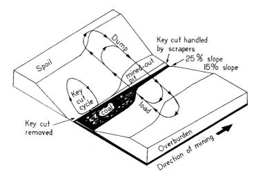
Fig.5.7. Block area/dozer-scraper method (after Ryan, 1982)
