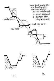
Fig.5.30. Haul road geometric considerations, a. haul road outside ore body, b. Haul road in ore body (after Atkinson, 1992)
