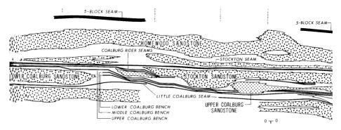
Fig.6.19. Geologic cross section of exemplary deposit (after Tussey, 1992)
