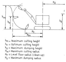
Fig.5.16. Essential dimensions of loading shovels (after Atkinson, 1992)
