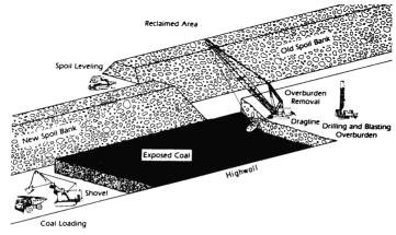
Fig.2.1. Surface mining, open cast method (after Anon, 1982)
