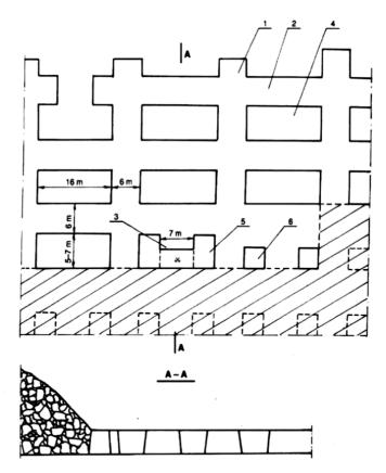
Fig.8.10. One-phase room-and-pillar method with roof caving (after Cieślik et al, 1991) 1. room; 2. strip; 3. cut into gob area; 4. pillar; 5. supporting (resistant) block (pillar); 6. ripped supporting pillar
