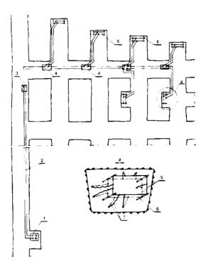
Fig.8.19. Electrical circuits for group firing of faces with parallel-series connection of electric detonators (after Janowski et al, 1996)
