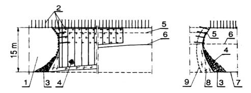
Fig.8.16. Supporting for roof and walls in high inclined drifts (after Cieślik et al, 1991)
