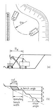
Fig.5.15. Double-spot loading and machine excavation group (R<sub>d</sub> is maximum dumping radius) (after Atkinson, 1992)
