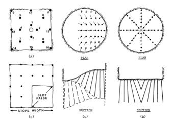
Fig.3.7. Single face drilling patterns for (A) a long-hole raise, (B) drop raise for blasthole stopes, (C) shaft bench round, and (D) full face V shaft round (after Dowding and Aimone, 1992)
