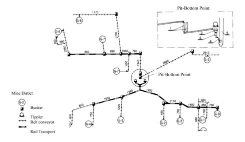
Fig.8.29. Transport of excavated ore with a combination of belt conveyor and rail transport (after Gładysiewicz and Pelc, 1996)
