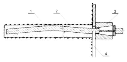
Fig.8.38. Rope bolt with cement (after Janowski et al, 1996) 1.rope rod; 2. cement; 3. clamp; 4. washer
