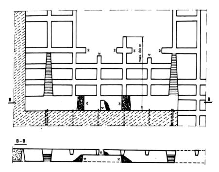
Fig.8.15. Two-layer room-and-pillar method with hydraulic backfilling (after Cieślik et al, 1991)
