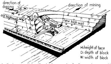
Block-digging operation with wheel excavator feeding on to a movable conveyor belt
