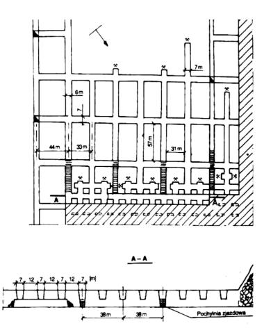
Fig.8.13. Two-layer room-and-pillar method with roof caving (after Cieślik et al, 1991)
