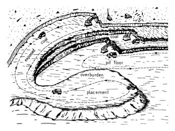
Fig.5.6. Modified open pit: flat-lying seams (after Anon, 1975)
