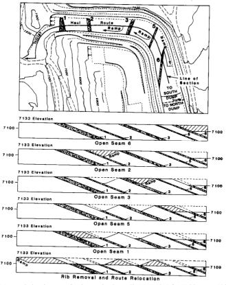
Fig.6.5. Bench development for the south wingwall, 1-UD pit (after Whitmann, 1992)
