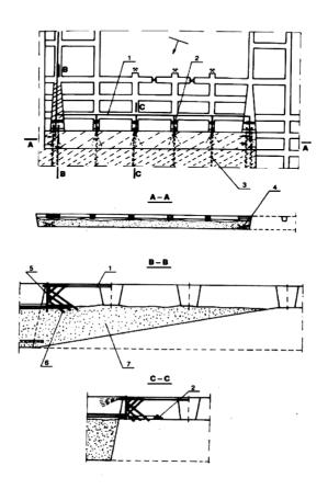
Fig.8.18. Mined-out area (goaf) backfilling (after Cieślik et al, 1991) 1. hydraulic stowage pipeline; 2.stoppings; 3. pipe channels; 4. filtration pipeline; 5. screen; 6. stretchers in sand floor on the floor bars; 7. backfilled inclined drift
