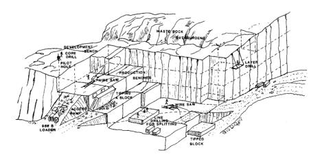
Fig.6.7. Schematic representation of quarry development (after Meade, 1992)
