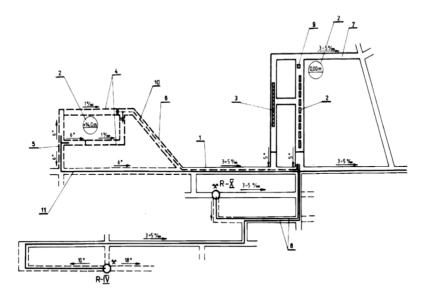
Fig.8.42. Main mine drainage system in Rudna mine (after Duda and Adamek, 1996) 1. roadway; 2. main drainage pump chamber, pumping the water directly onto the surface; pumping height 980 m; flow height 14,0m; 3switching station; 4. water tanks; 5. delivering water from deep parts of mine; 6. pipelines; 7. air roadway; 8. pumping pipelines to shafts; 9. cooling water; 10. pipeline; 11. pipeline
