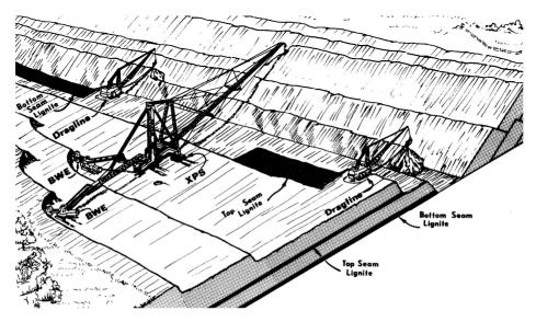
Fig.6.22. Cross-pit spreader and dragline combination C area (after Rand, 1992)
