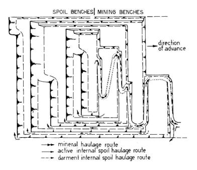
Fig.5.28. Diagrammatic terrace mine layout (after Atkinson, 1992)
