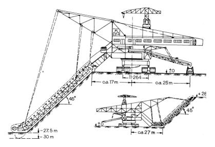
Fig.5.21. Bucket chain excavator (after Atkinson, 1992)
