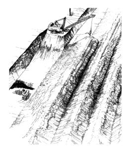
Fig.6.9. Conventional area mining utilizing a dragline (after Anon, 1979)
