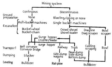
Fig.5.14. Materials handling system classification diagram (after Atkinson, 1992)
