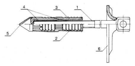
Fig.8.36. Wedge-and-sleeve bolt with load-bearing capacity of 150 kN (after Janowski et al, 1996) 1. rod; 2. head; 3. jaw; 4. expanding wedge; 5. cone cap; 6. resistant washer
