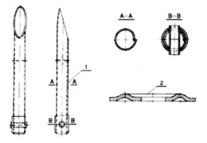
Fig.8.39. Tube-abrasive bolt (after Janowski et al, 1996)
