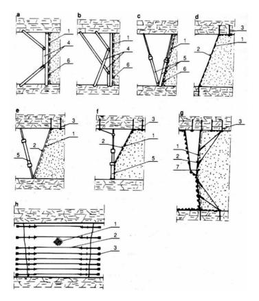
Fig.8.9. Schematic diagram of the construction of screens (backfilling stoppings) used in Polish copper mines (after Janowski et al, 1996)
