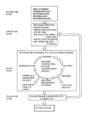
Fig.5.1. Diagrammatic presentation of the design process (after Fourie, 1992)
