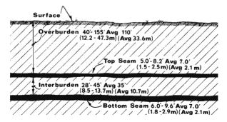
Fig.6.20.Cross section of C area (after Rand, 1992)
