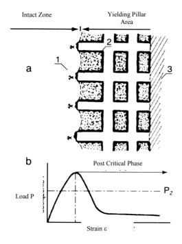
Fig.8.1.Schematic of one phase room-and-pillar mining system (a) simplified characteristics of the technological pillar behaviour (operation) (b) (after Kunysz et al, 1996)
