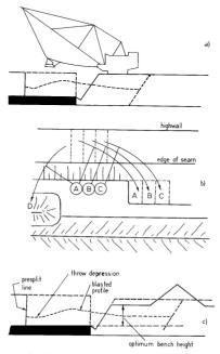
Fig.5.12. Cross-pit, chop-down with single seam (after Atkinson, 1992)
