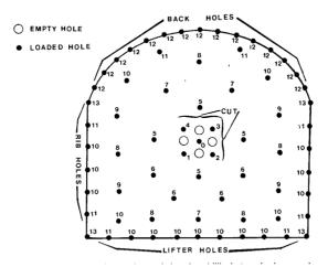
Fig.3.5. Typical tunnel round showing drillhole terminology and an initiation sequence for delay timing; all holes between the cut and perimeter holes are referred to as relief holes (after Dowding and Aimone, 1992)
