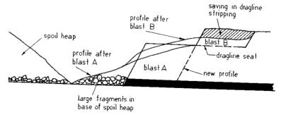
Fig.5.8. Throw blasting for a standard dragline operation (after Atkinson, 1992)
