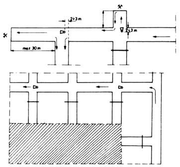
Fig.8.32. Ventilation of roadways by means of ventilating ducts (air ducts) (after Wacławik et al, 1996)
