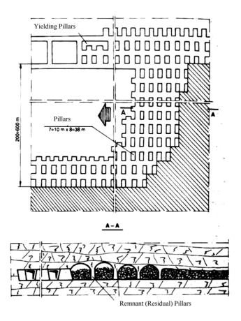
Fig.8.11. One-phase room-and-pillar method with retarded caving (roof deflection) (after Cieślik et al, 1991) 8.2.2 Room-and-Pillar Mining Methods with Roof Caving for Deposits with Thickness Greater than 5m
