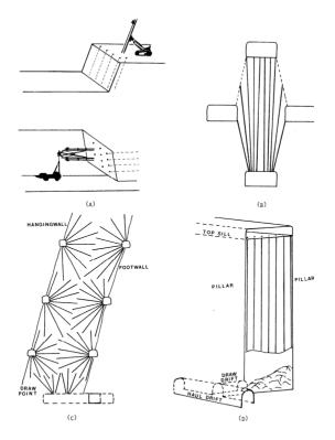
Fig.3.8. Multiple face drilling patterns for (A) room and pillar, cut and fill, and shrinkage stoping methods; (B) sublevel caving; (C) sublevel stoping; and (D) long-hole stoping or vertical crater retreat methods (after Dowding and Aimone, 1992)
