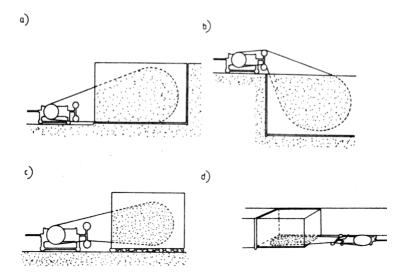
Fig.6.6. Cutting with a diamond line sawing machine
