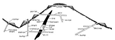
Fig.2.2.Underground mining, stoping method (after Anon, 1983a)
