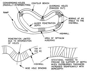
Fig.6.24. Trench-strip mining with the extended depth highwall mining system (after, Treuhaft, 1984)
