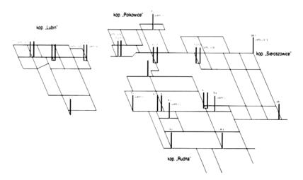
Fig.8.30. Spatial lay-out of the main ventilation system (after Wacławik et al, 1996)
