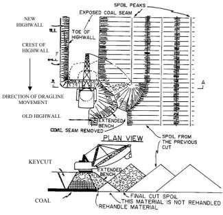
Fig.6.13. Extended bench stripping (after Bricker, 1992)
