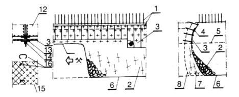
Fig.8.17. Supporting of roof and walls in high mining rooms (after Cieślik et al, 1991) 1. resin-bedded bolts; 2. screen; 3. wire mesh; 4. floor of hard rocks; 5. floor of upper layer; 6. floor of lower layer; 7. wall scaling zone; 8. wall cracking zone boundary; 12. mesh mounting; 13. pad; 14. nut; 15. mesh joining;16. fastener for mesh elements
