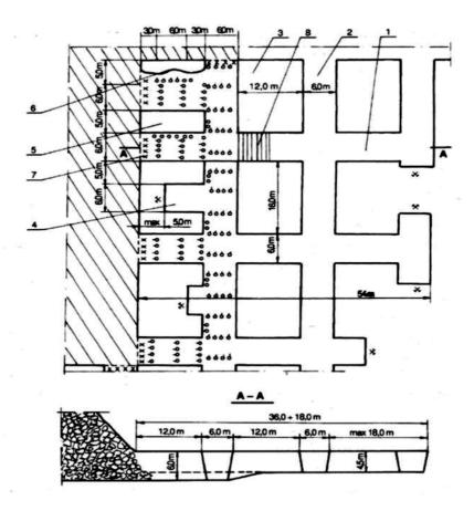
Fig.8.12. One-phase room-and-pillar method with roof caving (after Cieślik et al, 1991) 1. room; 2. strip; 3. pillar; 4. room for caving; 5. supporting block; 6. insets (cuts); 7. retaining partition; 8. inclined drift
