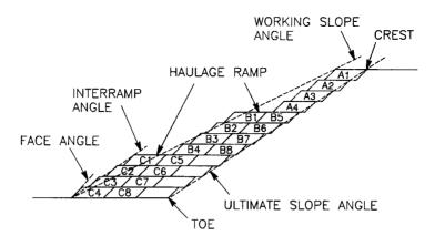
Fig.6.1. Cut sequence for sequential pushbacks (after McCarter, 1992)
