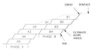
Fig.6.2. Cut sequence for conventional pushbacks (after McCarter, 1992)
