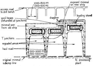
Fig.5.27. Diagrammatic strip mine layout (after Atkinson, 1992)
