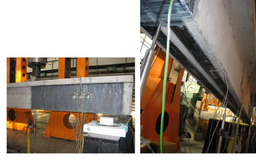
Fig. 2. Support zone of strengthened beam no. 2
