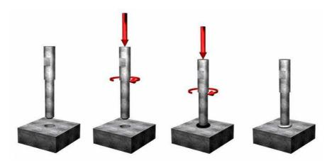
Fig. 1. Schematic illustration of FHPP
