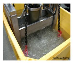
Fig. 3. System for underwater friction welding
