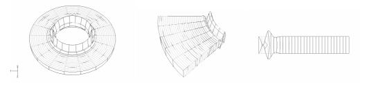
Fig. 13. Buckling of plate modelled as full annulus
