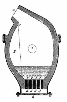
and all communicating with the space d d, into which opens the blast tube from a powerful blowing engine. The number of these blast holes varies from fifty or sixty to a hundred or more, according to the size of the converter.
