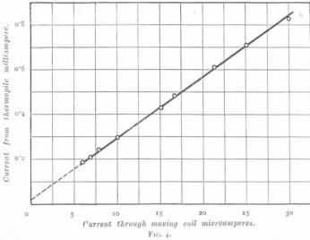
red. In intermediate positions the current generated by the thermopile is nearly proportional to the deflection.
