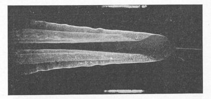
FIG. 3.-Low velocity type of flow. Water.
