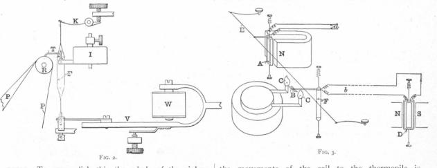
paper. To accomplish this the whole of the siphon suspension is vibrated rapidly up and down between the springs V and K by means of the spring V, which is attached to the vibrator. As the spring V is very weak in comparison with the reed, the vibrations of the latter are not affected by the movements of the spring. To impart a jerk to the siphon a stop, H, is fixed directly under the axis of suspensions, and two little dash-pots, DD, on either side prevent the spring bouncing on the stop.
