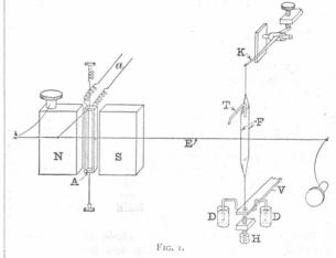
diameter. The moving coil consists of 500 turns of 2-mil wire at a mean radius of  $\frac{3}{8}$  in. The coil and siphon are mounted on separate axes and are connected by silk fibres so that the angular movement of the siphon is about two to three times that of the coil. By reducing the length of the siphon to  $\frac{1}{2}$  in. and substituting a narrower coil it is possible greatly to increase the sensitiveness of the recorder.
