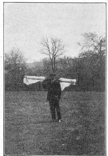
FIG. 3.—Kite folded for carrying.
