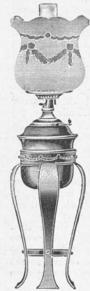
FIG. 1.—“Petrolite” lamp using upright incandescent mantle fed by air which has passed through porous material impregnated with volatile hydrocarbons.
