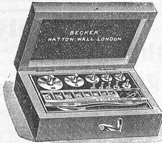
N 2306.—F. E. Becker & Co.'s Analytical Weights, some of the fractions made of 18 ct. gold.
