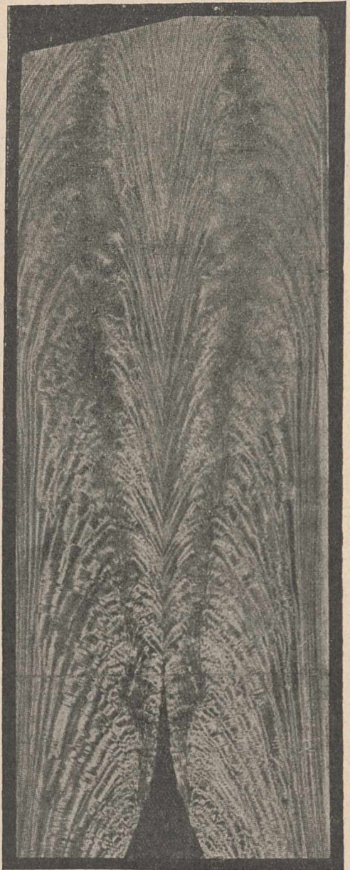
Fine example of African mahogany curl. (From "A Manual of the Timbers of the World.")
