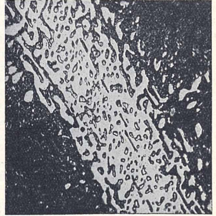
FIG. 2.—Eutectic-like appearance of cementite. \times 500 .
