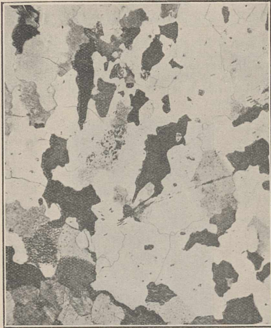
FIG. 1.—Microstructure of pure mercury. Magnification: \times 100 .
