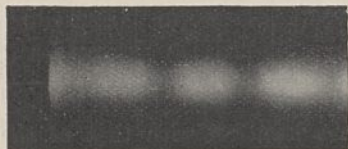
FIG. 1.—Pressure, 0.4 mm.; diameter of tube, 2.9 cm.; distance between electrodes, 11.5 cm.; \lambda=80 metres.
