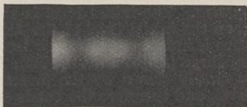
FIG. 2.—Pressure, 0.4 mm.; diameter of tube, 2.9 cm.; distance between electrodes, 6 cm.; \lambda=80 metres.
