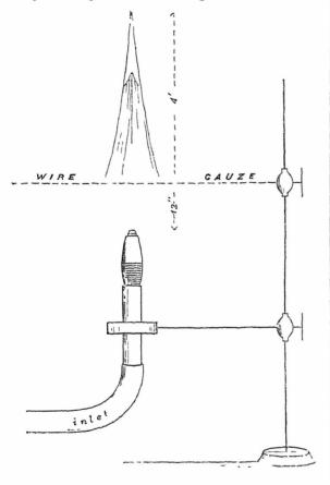
inches square, resting on the ring of the retort-stand—ordinary window-blind wire-gauze 32 meshes to the lineal inch. The burner was Sugg's steatite pin-hole burner, the same as used for vowel flame.
