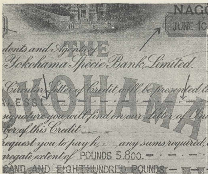
FIG. 1. Fluorescence photograph of a forged document. Arrows indicate original wording, which is not visible in daylight.
