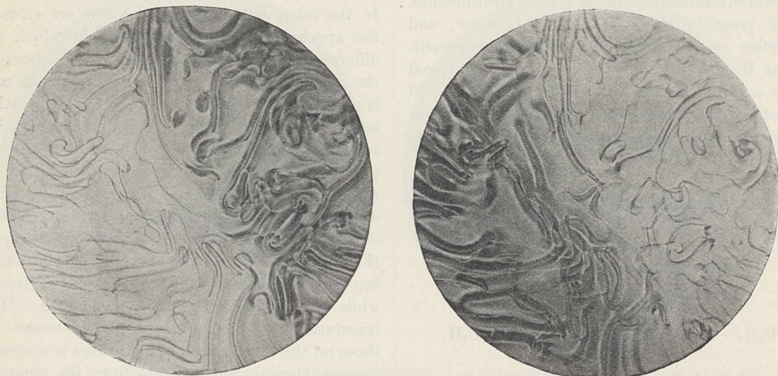
FIG. 13.—The two photographs show the same substance, para -azoxyphenetole in the nematic phase, at two moments separated by as short an interval as possible. The only difference is that the position of the analyser in one case is approximately at right angles to its position in the other. No polariser. The clearer portion of each photograph is seen by ordinary rays; and the other by extraordinary rays.
