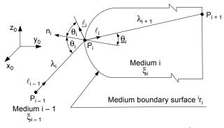
Fig. 2. Skew ray tracing at medium boundary surface  ${}^{i}r_{i}$ .
