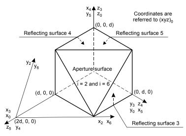
Fig. 3. Coordinate frames used to define flat boundary surface of solid glass corner-cube.
