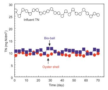
Fig. 5. Total nitrogen concentration in treated effluent of the BAF systems
