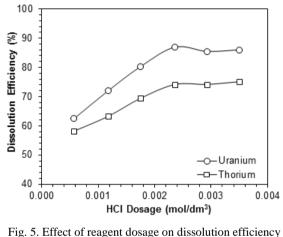
of uranium and thorium from the fly ash sample (30% solid concentration, 240 min leaching time, temperature 20 °C)
