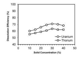
Fig. 3. Effect of solid concentration on dissolution efficiency of uranium and thorium from the fly ash sample (1.18 mmol/dm<sup>3</sup> HCl, 240 min leaching time at 20 °C, pH~2.79)
