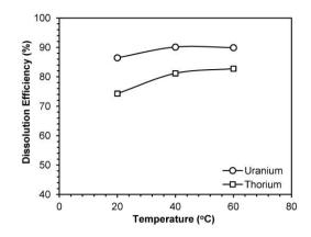
Fig. 6. Effect of temperature on dissolution efficiency of uranium and thorium from the fly ash sample (2.36 mmol/dm<sup>3</sup> HCl, 30% solid concentration, 240 min leaching time, pH~2.77)
