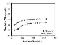
Fig. 4. Effect of leaching time on the dissolution efficiency of uranium and thorium from the fly ash sample (1.18 mmol/dm<sup>3</sup> HCl, 30% solid concentration, temperature 20 °C, pH~2.81)
