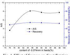
Fig. 4. Effect of fineness on direct flotation (NaOl 800 g/Mg, Na<sub>2</sub>CO<sub>3</sub> 3000 g/Mg, Calgon 60 g/Mg)
