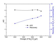
Fig. 5. Effect of Na<sub>2</sub>CO<sub>3</sub> on direct flotation (-0.074mm 90%, NaOl 800 g/Mg, Calgon 60 g/Mg)
