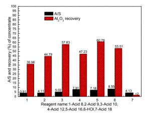
Fig. 8. Flotation results using straight chain alkyl fatty acid as collectors
