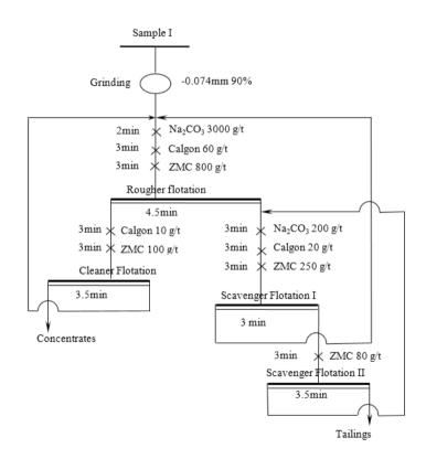
Fig. 11. Direct flotation tests for the Xinmi Mine ore (sample I) using ZMC collector (symbol g means gram while symbol t mean megagram)
