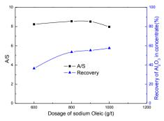
Fig. 7. Effect of sodium oleate on the direct flotation (-0.074 mm 90%, Na<sub>2</sub>CO<sub>3</sub> 3000 g/Mg, calgon 60 g/Mg)
