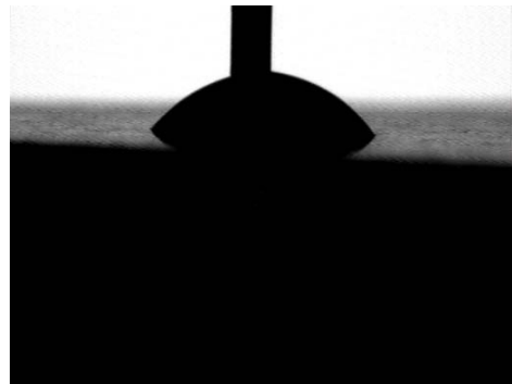
Fig. 2. Example of advancing contact angle measurement
