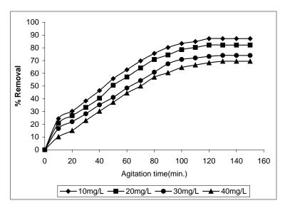
Fig. 2. Effect of agitation time and initial Pb(II) concentration on Pb(II) adsorption (adsorbent dosage: 50 mg/50 cm<sup>3</sup>, Pb(II) concentration: 10–40 mg/dm<sup>3</sup>)
