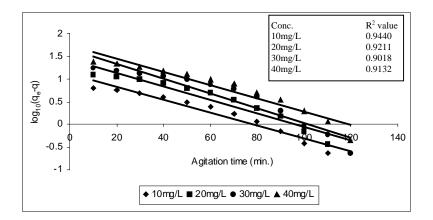
Fig. 3. Lagergren plots for Pb(II) adsorption (adsorbent dosage: 50 mg/50 cm<sup>3</sup>, Pb(II) concentration: 10–40 mg/dm<sup>3</sup>)
