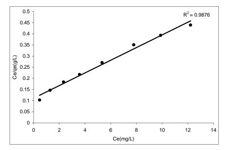
Fig. 5. Langmuir plot for Pb(II) adsorption (adsorbent dosage: 50 mg/50 cm<sup>3</sup>, Pb(II) concentration: 5–40 mg/dm<sup>3</sup>)
