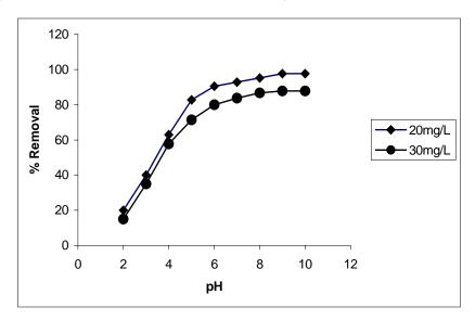
Fig. 7. Effect of pH on Pb(II) adsorption (adsorbent dosage: 50 mg/50 cm<sup>3</sup>, Pb(II) concentration: 20 and 30 mg/dm<sup>3</sup>)
