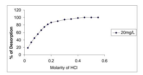
Fig. 8. Desorption of Pb(II) ions from RCP carbon
