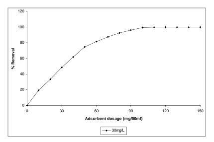
Fig. 4. Effect of carbon dosage on Pb(II) adsorption (adsorbent dosage: 0–150 mg/50 cm<sup>3</sup>, Pb(II) concentration: 30 mg/dm<sup>3</sup>)
