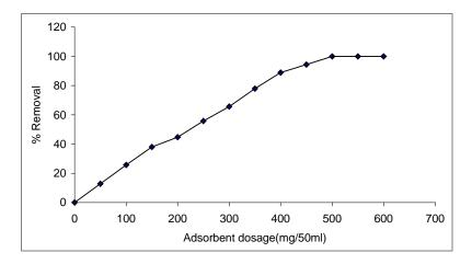
Fig. 9. Effect of carbon dosage on lead removal from industrial wastewater (adsorbent dosage: 50–600 mg/50 cm<sup>3</sup>, Pb(II) concentration: 30 mg/dm<sup>3</sup>)
