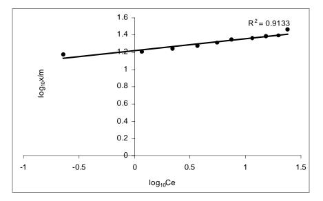
Fig. 6. Freundlich plot for Pb(II) adsorption (adsorbent dosage: 50 mg/50 cm<sup>3</sup>, Pb(II) concentration: 5–40 mg/dm<sup>3</sup>)
