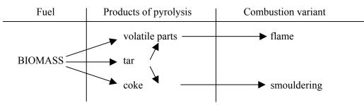
Combustion technology and conditions, furnace construction and fuel quality affect the composition of pollutants emitted during wood combustion. Apart from stove design parameters, combustion emissions are first of all dependent on adequate excess air and fuel parameters.
