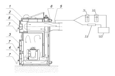
Scheme of boiler with retort furnace, including description of its components and diagram of sampling system:
