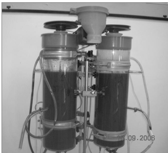
Fig. 1. Laboratory reactors for biological sewage treatment
