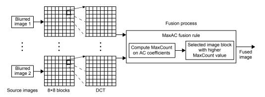
Fig. 1. General structure of the proposed fusion scheme.
