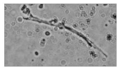
Photo 1. A standard asbestos fibre with characteristically sharp edges in one of the samples
