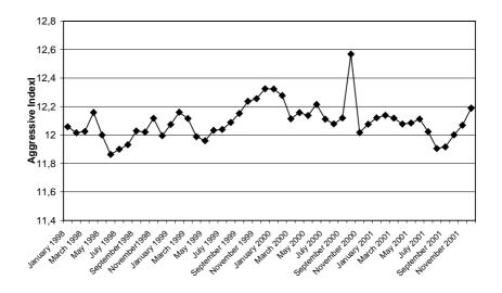
Fig. 4. Aggressive Indices calculated for finished water produced by the Bielany WTP (the Sanka River) – based on data provided by the local waterworks company
