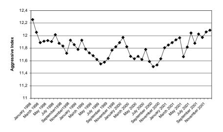
Fig. 1. Aggressive Indices calculated for finished water produced by the Dobczyce Reservoir WTP – based on data provided by the local waterworks company
