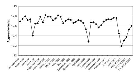
Fig. 3. Aggressive Indices calculated for finished water produced by the Dłubnia Reservoir WTP – based on data provided by the local waterworks company
