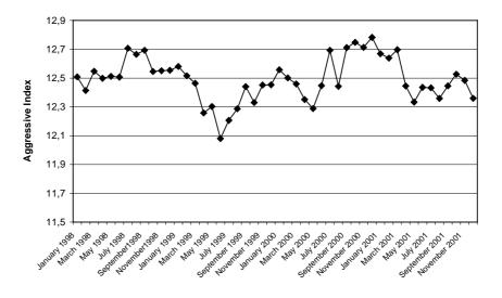
Fig. 2. Aggressive Indices calculated for finished water produced by the Rudawa River WTP – based on data provided by the local waterworks company
