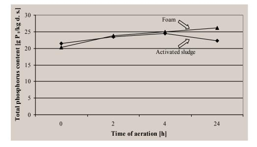
Fig. 1. Concentration of total phosphorus in activated sludge biomass and filamentous microorganisms versus aeration time
