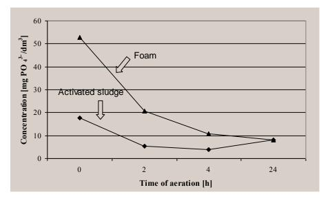
Fig. 2. Concentration of phosphates in the liquid associated with activated sludge and foam versus time of aeration
