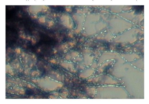
Phot. 3. Polyphosphate granules in the filamentous microorganisms - contrast-phase microscope
