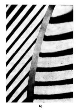
Fig. 7. Images of a glass plate in the Twyman-Green interferometer with laser illumination: a) without noise elimination, b) with a rotating block
