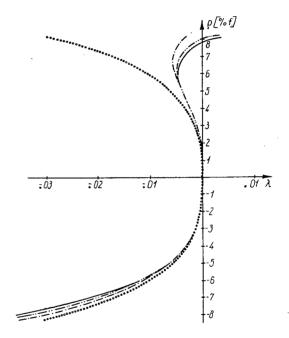
Fig. 1c. The graphs of the wave aberration for the field angle 12°
