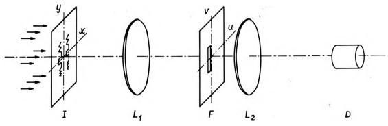
Fig. 1. Double-slit arrangement according to method 1 I – input plane,  $L_1$  – transform lens, F – Fourier plane,  $L_2$  – collecting lens, D – detector
