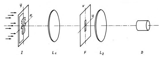
Fig. 2. One-dimensional Fourier transform subtraction arrangement according to method 2 I – input plane,  $L_1$  – transform lens, F – Fourier plane,  $L_2$  – collecting lens, D – detector
