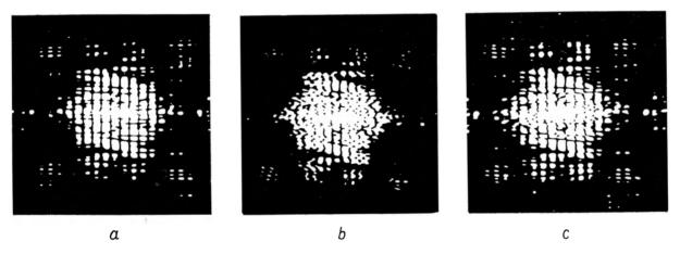
Fig. 3. Diffraction patterns of (a) standard, correctly adjusted profile, (b) standard, slightly rotated profile, (c) faulty profile
