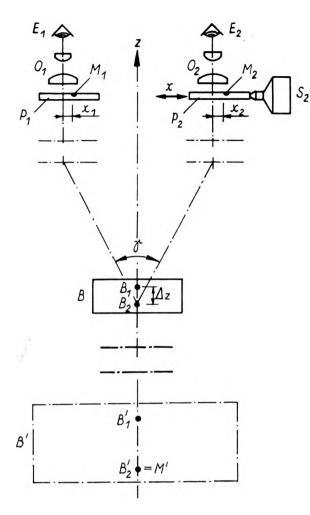
Fig. 1. Schematic diagram showing the principle of stereoscopic depth measurements under the microscope
