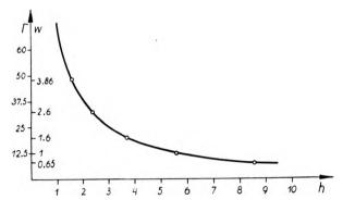
Fig. 2. Dependence between the factor h and total magnifying power  $\Gamma$  (or magnification coefficient W) for a typical stereoscopic microscope
