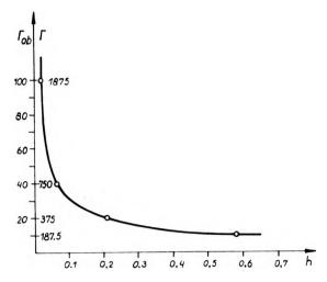
Fig. 4. Dependence between the factor h and total magnifying power  $\Gamma$  of the mono-objective phase contrast stereoscopic microscope MB30S ( $\Gamma_{\rm ob}$  - objective magnification)
