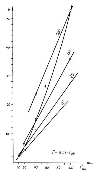
Fig. 5. Parameter k plotted against the total magnification  $\Gamma$ and condenser aperture of the mono-objective phase contrast stereoscopic microscope MB30S
