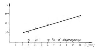
Fig. 6. Dependence between the parameter k and diameter D of annular condenser diaphragms of the mono-objective phase contrast stereoscopic microscope MB30S (objective 100x/1.3)
