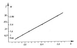
Fig. 3. Parameter k plotted against the total magnifying power  $\Gamma$  (or magnification coefficient W) of a typical stereoscopic microscope
