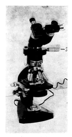
Fig. 7. Photograph of the mono-objective phase contrast stereoscopic microscope MB30S fitted with the microstereometric device described in the text
