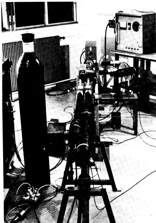
Fig. 8. Disposition of optical elements and detectors in the apparatus for measurements of weak Kerr birefringences during the first microsecond of external electric field action
