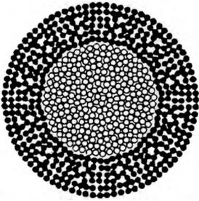
Fig. 3. Cross-section of concentric version of transmitting/receiving bundle (computer processed):  $\circ$  — transmitting optical fibers,  $\bullet$  — receiving optical fibers.
