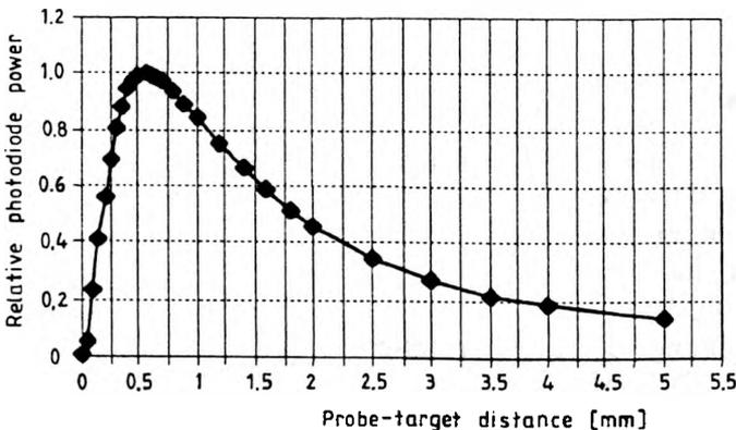
Fig. 4. Relative photodiode power versus probe to target distance for concentric version of transmitting/receiving bundle.
