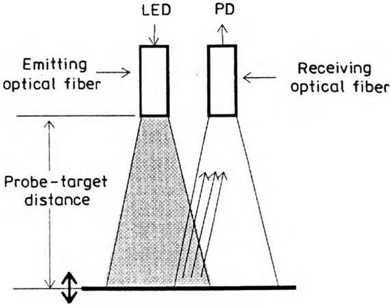
Fig. 1. Fiber vibrometer operating principle.
