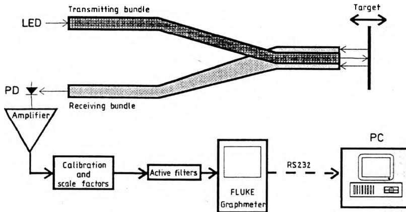
Fig. 5. Layout of the fiber vibrometer.
