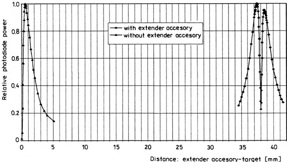
Fig. 9. Relative photodiode power versus probe-target and/or extender accessory-target distance. Note a considerable increase of the operating distance obtained using the extender accessory.
