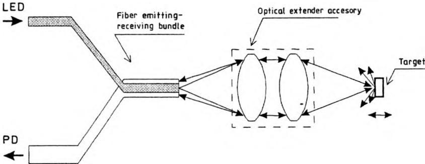
Fig. 8. Fiber vibrometer with optional extender accessory.
