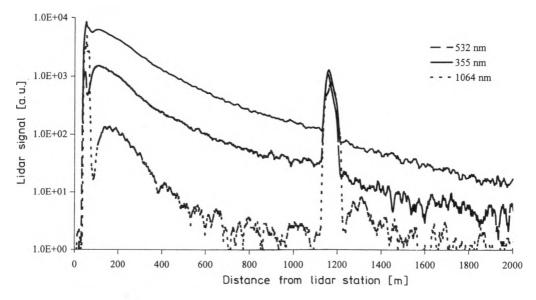
Fig. 7. Lidar echoes from the stack emission plume at three different laser wavelengths.
