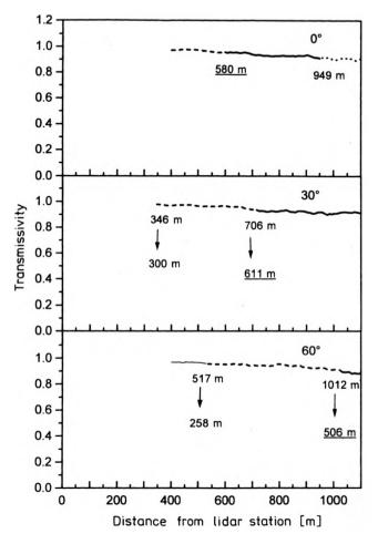
Fig. 4. Transmissivity profiles at three different zenithal angles. The same range in the vertical direction has been indicated by the same line type. The arrows indicate the corresponding height along the vertical direction.
