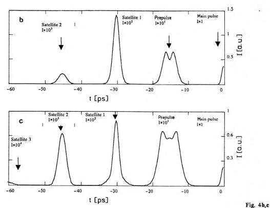
Fig. 4. Increase of prepulses under following initial conditions: duration of chirped pulses -1 ns, compressed pulses -1 ps, delay between main pulse and prepulse -15 ps, main pulse to prepulse intensity ratio -10 times, value of *B*-integral: 0.5 (a), 3 (b), 5 (c)
