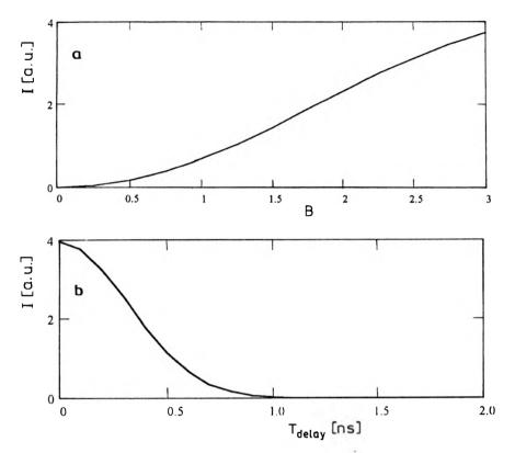
Fig. 3. Increase of first satellite intensity with B-integral under conditions of Fig. 2 (a). Decrease of first satellite intensity with time delay between main pulse and postpulse under conditions of Fig. 2 (b).
