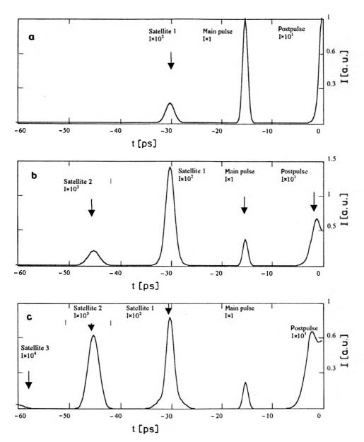
Fig. 2. Arise and increase of prepulses under following initial conditions: duration of chirped pulses -1 ns, compressed pulses -1 ps, delay between main pulse and postpulse -15 ps, main pulse to postpulse intensity ratio -10 times, value of B-integral: 0.5 (a), 3 (b), 5 (c).
