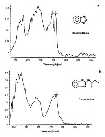
Fig. 3. The UV spectra of: 0.5 mg/L benzimidazole in CH<sub>3</sub>CN (a) and 0.7 mg/L carbendazime in CH<sub>3</sub>CN (b).
