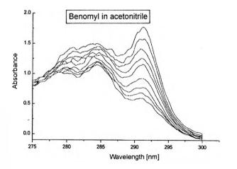
Fig. 4. The 2D UV spectra of 0.65 mg/L benomyl in CH<sub>3</sub>CN for different periods of time.
