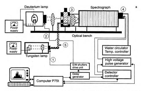
1, 2 - electromechanical shutters, 3 - sample cell holder, 4 - CCD optical detector, 5 - optical fiber
