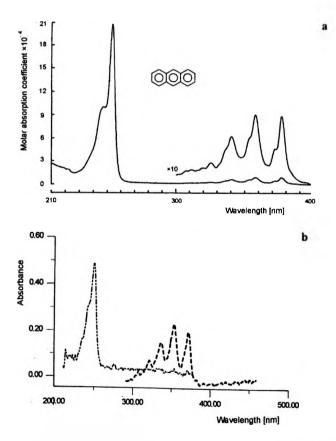
Fig. 2. Absorption spectrum of 0.73 mg/L anthracene in cyclohexane as obtained in reference [8] using Perkin-Elmer Model 555 instrument –  $\mathbf{a}$ , absorption spectrum of the same concentration as in  $\mathbf{a}$  obtained by the new system –  $\mathbf{b}$ .
