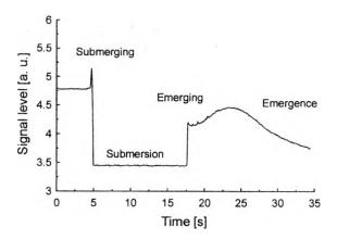
Fig. 2. Full measuring cycle in the time domain for eatable oil sample.
