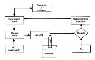
Fig. 1. Block diagram of automatic sensor.
