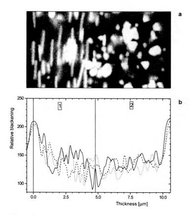
Fig. 1. Microscopic image of a cross-section of the light sensitive layer of Kodak T-max 400 negative. Magnification  $5000 \times$  (a). Averaged profile of relative blackening in the image of the cross-section of the light sensitive layer of Kodak T-max 400. 1 – fluctuation area corresponding to surface component sublayer containing tabular crystals of AgHal, 2 – sublayer containing spherical crystals (b).
