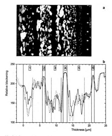
Fig. 3. Microscopic image of the cross-section of the light sensitive layer of the Fujicolour Superia 200 colour negative. Magnification  $2000 \times$  (a). Averaged image blackening profile for light-sensitive layer cross-section of the Fujicolour Superia 200. 1, 3, 5 – fluctuation areas corresponding to main component layers: blue-, green- and red-sensitive ones. Fields 2 and 4 correspond to intermediate layers while field 6 – to the antihalo layer (b).
