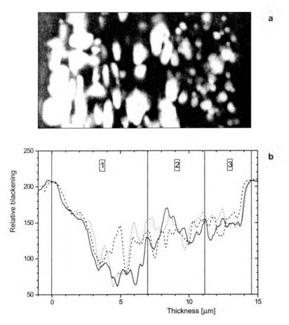
Fig. 2. Microscopic image of the cross-section of the light-sensitive layer of the Konica Monochrome VX 400 negative. Magnification  $5000 \times$  (a). Averaged image blackening profile for light-sensitive layer cross-section of Konica Monochrome VX400. 1, 2, 3 — fluctuation areas corresponding to the layers of the light-sensitive emulsion differing from each other by the magnitude of the spherical crystals of AgHal (b).
