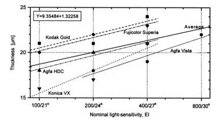
Fig. 4. Relation between the total thickness of the light sensitive emulsion layer and the nominal exposure index determined for a group of light-sensitive materials under examination.
