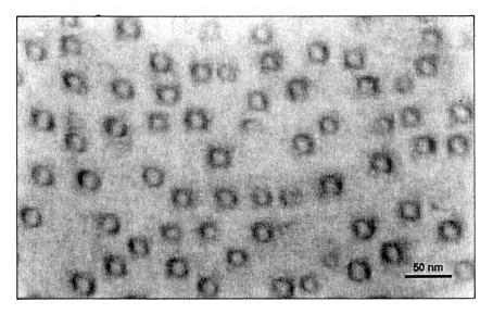
Fig. 1. Plane-view TEM image in [001] direction of InGaAs QDs embedded in GaAs matrix. The diameter of QDs is approximately 20-30 nm and their surface density is  $4.5 \times 10^{10}$  cm<sup>-2</sup>.
