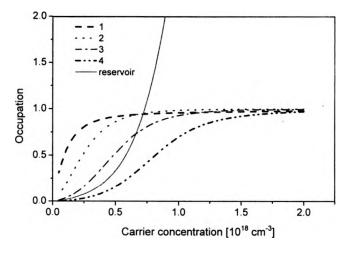
Fig. 6. Population of dot states  $E_n$ ,  $n = 1, \dots, 4$  as a function of external excitation density at 300 K.
