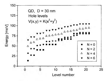
Fig. 5. Hole energy levels in InAs/GaAs QD calculated by the self-consistent Hartree method for different dot occupations (n - level number, N - number of electrons in QD).
