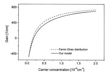
Fig. 7. Gain for the transitions between n = 1 levels in QD as a function of external excitation density at 300 K.
