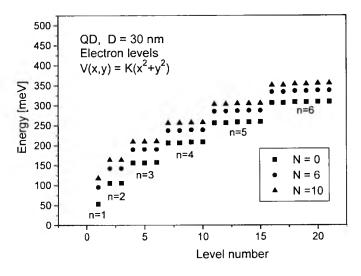
Fig. 4. Electron energy levels in InAs/GaAs QD calculated by the self-consistent Hartree method for different dot occupations (n – level number, N – number of electrons in QD). V(x,y) – quantum dot harmonic potential,  $K = 3 \cdot 10^{14}$  V/m<sup>2</sup>.
