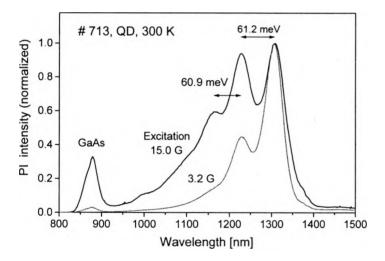
Fig. 3. Spontaneous emission vs. wavelength at 300 K for different excitation intensities.
