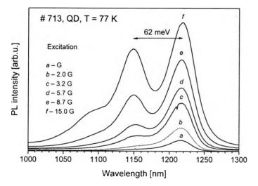
Fig. 2. Spontaneous emission vs. wavelength at 77 K for different excitation intensities (G – excitation density,  $G = 10^5$  W/m<sup>2</sup>).
