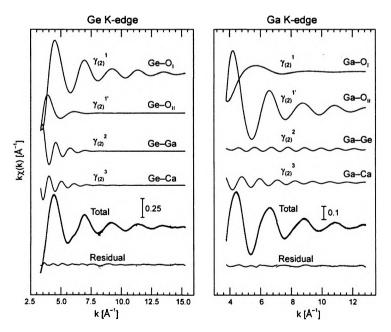
Figure 3. Results of the GNXAS analysis performed for spectra recorded at Ge and Ga-edges of  $Ca_3Ga_2Ge_4O_{14}$  glass (solid line – model; dotted – experiment). See also Tab. 2
