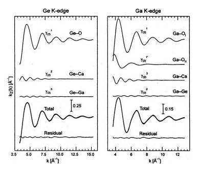
Fig. 2. Results of the GNXAS analysis performed for spectra recorded at Ge and Ga-edges of  $Ca_3Ga_2Ge_3O_{12}$  glass (solid line – model; dotted – experiment). See also Tab. 1.
