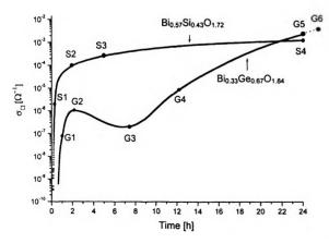
Fig. 1. Time dependence of surface conductivity of Bi<sub>0.33</sub>Ge<sub>0.67</sub>O<sub>1.84</sub> and Bi<sub>0.57</sub>Si<sub>0.43</sub>O<sub>1.72</sub> glasses during heat treatment at 613 K.
