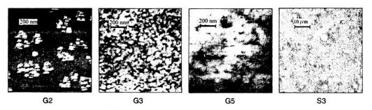
Fig. 2. AFM pictures of  $Bi_{0.33}Ge_{0.67}O_{1.84}$  (G2, G3 and G5) and  $Bi_{0.57}Si_{0.43}O_{1.72}$  (S3) glass samples.
