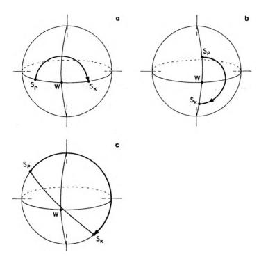
Fig. 1. Three most important cases of using the half-wave plates in optical setups: change of the azimuth angle of linearly polarized light (a); change of the sign of the ellipticity of light (b); change of the polarization state of light into perpendicular one (c).
