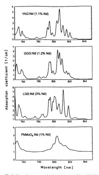
Fig. 3. Absorption spectrum for Nd:GGG, Nd:LGS and Nd:PbMoO<sub>4</sub> compared with Nd:YAG at laser diode pumped region of 750-850 nm
