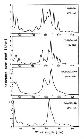
Fig. 1. Absorption spectrum for Nd:YAlO<sub>3</sub>, Nd:SrLaGa<sub>3</sub>O<sub>7</sub> and Nd:SrLaAlO<sub>4</sub> compared with Nd:Y<sub>3</sub>Al<sub>5</sub>O<sub>12</sub> for laser diode pumped region of 750-850 nm
