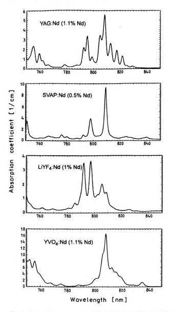
Fig. 4. Absorption spectrum for Nd:SVAP, Nd:YLF and Nd:YVO compared with Nd:YAG at laser diode pumped region
