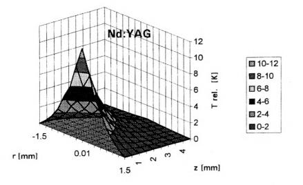
Fig. 5. Calculated cw temperature distribution in an optically end-pumped laser rod for the 1 W pump power. The heat source is assumed to be radially symmetric of Gaussian shape with constant radius along z-axis
