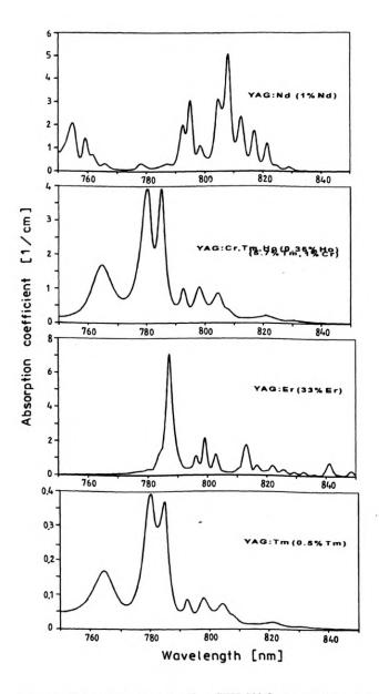
Fig. 2. Absorption spectrum for CTH:YAG, Er:YAG and Tm:YAG compared with Nd:YAG for laser diode pumped region of 750-850 nm
