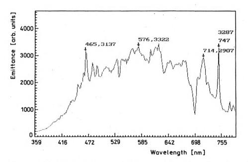
Fig. 2. Spectral remittance curve of the xenon-arc light source used for the measurement of the remittance spectra
