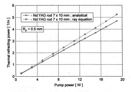
Fig. 1. Thermal refractive power versus pump power for Nd:YAG laser
