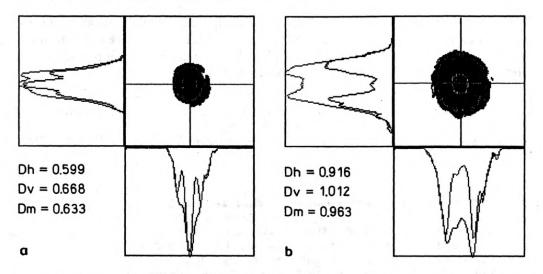
Fig. 7. Beam intensity distribution for the Nd:YAG laser:  $\mathbf{a}$  - Bessel-like shape at a distance of 480 mm from the lens,  $\mathbf{b}$  - annular-like shape at a distance of 520 mm from the lens
