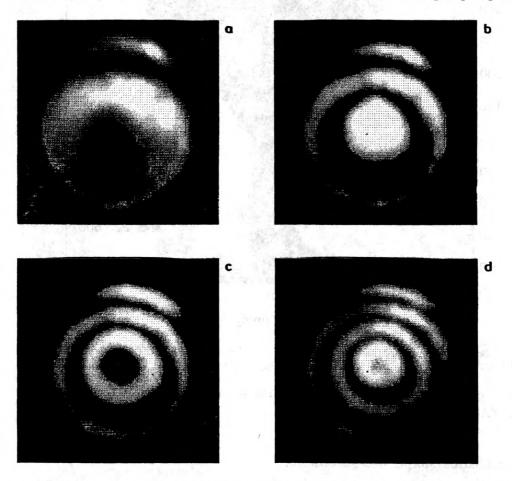
Fig. 4. Interferograms of thermally induced wavefront aberration of Nd: YAG rod  $7 \times 10$  mm for several values of pump power:  $\mathbf{a} - 2.7$  W,  $\mathbf{b} - 5.2$  W,  $\mathbf{c} - 7.5$  W,  $\mathbf{d} - 10.2$  W
