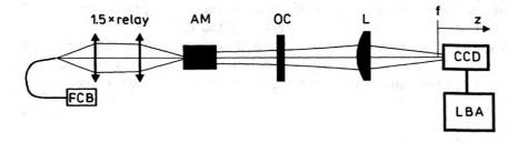
Fig. 5. Scheme of experimental setup: FCB – fiber coupled diode bar SDL3450-P5, AM – active medium (T-GRIN lens), OC – output coupler, L – lens, CCD – CCD camera Pulnix TM-745, LBA – laser beam analyser
