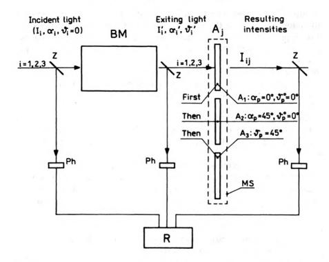
Fig. 2. Automatic system measuring the birefringent properties of the medium.  $I_i$ ,  $I'_i$ ,  $I_{ij}$  – light intensities,  $\alpha_i$ ,  $\alpha'_i$  – azimuths,  $\vartheta_i$ ,  $\vartheta'_i$  – ellipticity angles, EM – examined birefringent medium,  $A_j$  – analysers, MS – measuring system for polarization state determination, Ph – photodetectors, Z – mirrors, R – recording and data processing unit
