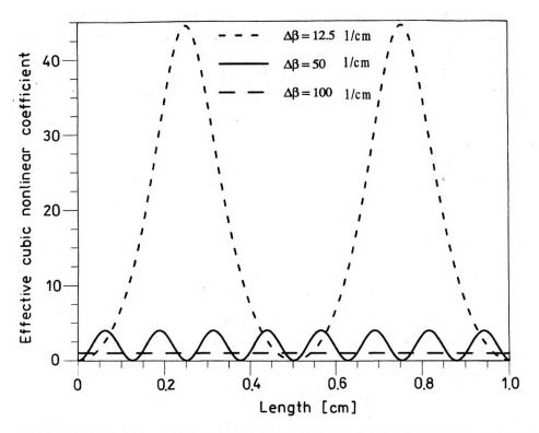
Fig. 2. Effective cubic nonlinear coefficient of the cascaded second-order process versus propagation length. Parameters: input irradiance 500 MW/cm<sup>2</sup>,  $d_{eff} = 3.1$  pm/V, n = 1.8,  $\lambda = 1.06$  µm
