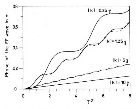
Fig. 1. Phase shift of the FF wave in the scalar ( $\delta = 0$ ) interaction for different ratios mismatch/nonlinearity as a function of the normalised length  $\xi = \gamma Z$  ( $\gamma = \text{const}$ ). Solid line – exact results, dashed line – approximation (7) used
