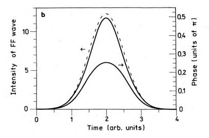
Fig. 4. Phase and amplitude modulation of a pulse with the input amplitude  $\gamma = \gamma_0 \exp(-\tau^2)$ . **a** - k = 0.25,  $\gamma_0 = 5.07$ , **b** - k = 4.3,  $\gamma_0 = 3.5$
