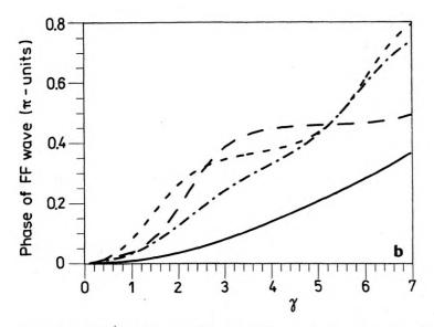
Fig. 3. Intensities (a) and phases (b) of the FF wave as a function of the nonlinearity  $\gamma = L\chi_{err}\sqrt{P}$ . The input is balanced ( $\delta = 0$ ); solid line: k = 17.3, dash-dotted line: k = 4.3, short-dashed line: k = 0.87, long-dashed line: k = 0.25
