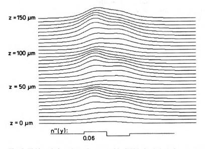
Fig. 5. Field evolution along the waveguide (BPM simulation), for  $\alpha < \alpha_{branch}$
