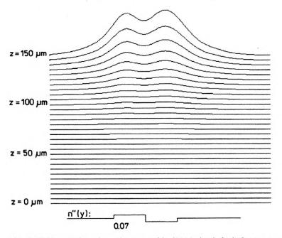
Fig. 6. Field evolution along the waveguide (BPM simulation), for  $\alpha > \alpha_{branch}$
